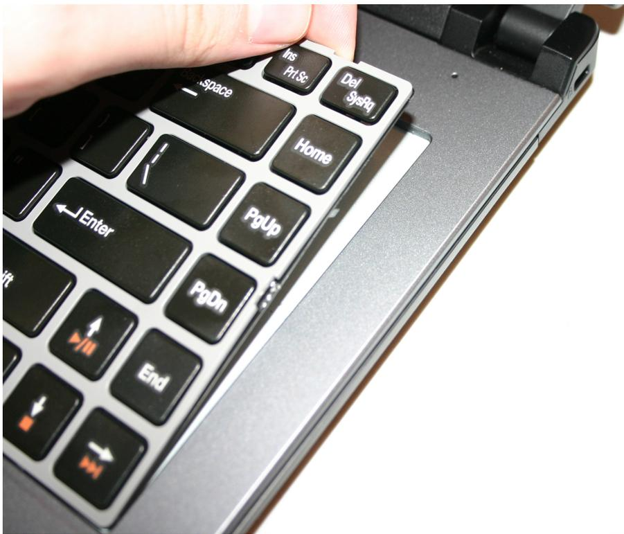
Lift keyboard. Use flat head screw driver to get “up” if needed. Be careful not to use force here.
