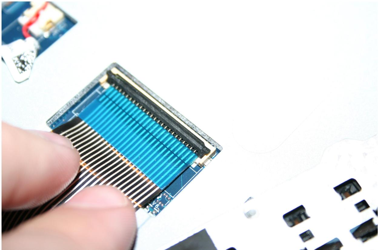
A picture after insertion of the keyboard's cable.
