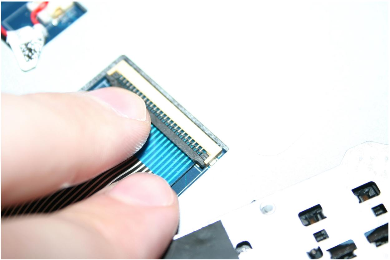
Press down on the black latch to secure cable.
