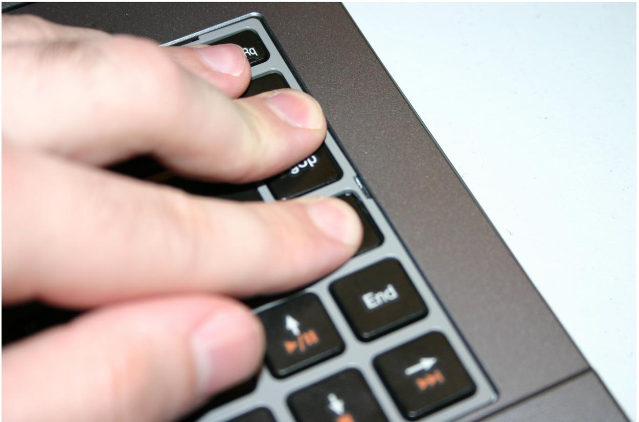
Secure the keyboard by pressing firmly around the edges.
