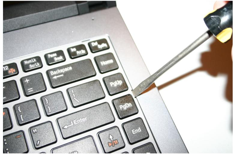
Using a flat head screw driver insert into the latch holes on keyboard. Press down to eject keyboard.
